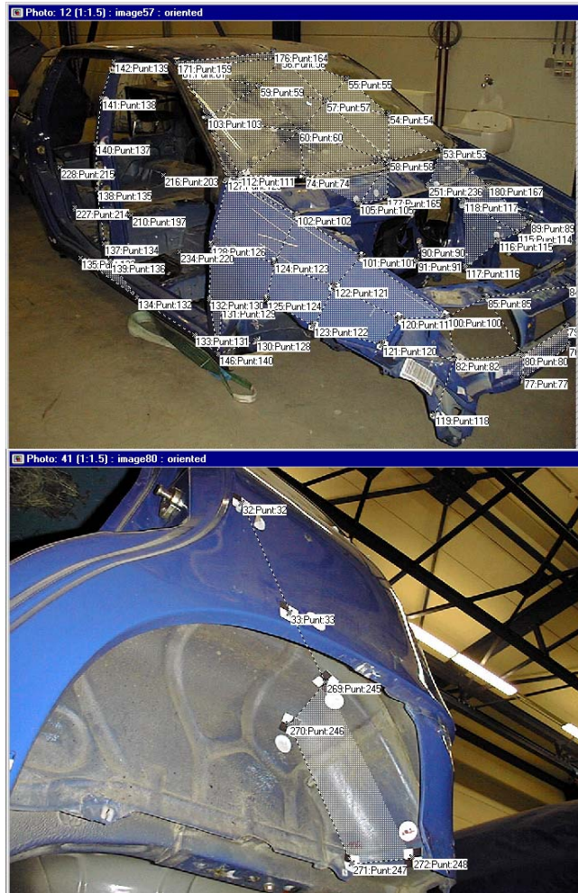
Figure 13 : photographs of the body in white with marked points, lables, lines and surfaces (full body and detail of wheel hub)
